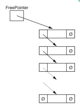
The following diagram shows an array of records that stores the tree shown in part (b).
